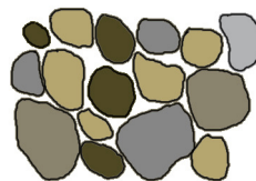
Compacted soil with greatly reduced pore space
